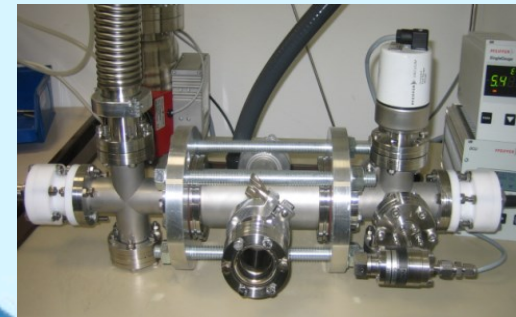
Sputtering system for the internal coating of tubes
